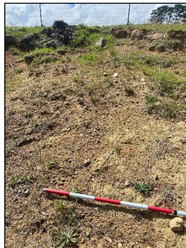
Plate 6. Dam cutting exposure with yellow clay and shale bedrock (east)
